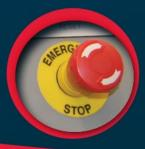
**E-Stop Functionality:** There are 3 different E-Stop switches that can be utilized in this system. There are two push-button stops, one on the operator console and the other located on the electrical panel. The third option is an emergency kick switch tied to the E-Stop system for quick, hands free use.
