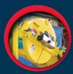
**Rotating Wheel Guard:** This allows the operator to move, re-align, and change castings safely without having to turn off the motor each time. The wheel guard technology includes sensors that are connected to a safety circuit. When pulling the handle down to start cutting the guard opens, allowing the operator to perform a cut.
