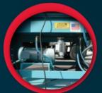
**Pneumatic/Vacuum System:** Foot operated electric control pedal for floatation to keep hands free for gondola movement. Pneumatics allow the gondola to float for easy movements; the vacuum system secures the gondola to the table during cutting.
