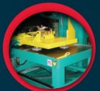
Air Float Table: Table is heavy-duty construction and Blanchard ground. The table can be turned over if worn or damaged, or completely replaced.
