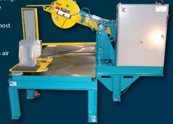
Hydraulic down force provides for quicker, cooler cuts with less blade wear. In all cases, the casting needs to be securely fixtured when using hydraulic down force. When using hydraulics we offer "On Demand" operation. This is where the saw is balanced and can be easily pulled down to make a scoring cut before hydraulic down force is applied.
