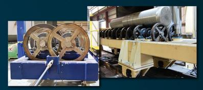
axel drives are available where space is limited. The rounds rotator can be equipped with "Easy Downs" to provide protection to the car, rotator wheels and drive shafts, recommended when loading equipment and procedures may allow the material to "drop" on the car.
