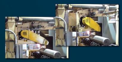
40 ft long). With the wheel oriented to an angle, the ends of the material can be chamfered. The lateral travel of the car is done with an electric drive and speeds can be maintained from 4 in per minute for spiral grinding to 200 ft per minute for longitudinal grinding. Auto-grinding and anti-penciling is also available.
