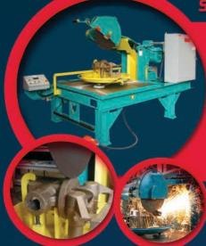
Standard Air Float Cut-Off machines offer the same convenience of using the gondola to easily move heavy castings, with manual saw movement. For more information such as photos, video and brochure, visit our website or scan the code below.
