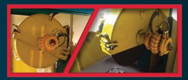
**Laser Alignment System:** Low-power laser mounted on the wheel guard for easy alignment of cut-off wheel. Laser is visible while operator has the vacuum system foot switch depressed.
